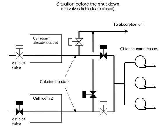
When the cell room 2 shut down, the "white" valve closed and the 2 "black" valves opened
